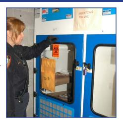
The PURAIR 30 Advance Ductless Fuming Hood was purchased and is used to protect technicians from exposure to harmful fumes during the processing of evidence for latent prints. This new equipment replaced a twelve year old chamber and is estimated to increase latent detection by twenty to thirty percent in cases involving hand guns, drug packaging materials and other items.
