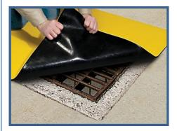
When vehicle washing is performed in the vicinity of a storm drainage collection system, cover the storm drain with a portable drain cover to prevent illegal discharges.
